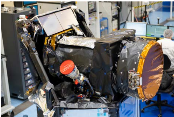
Figure 4: Picture of the payload after integration on the platform with the star tracker optical heads (red covers). Image credits Airbus DS Spain.
