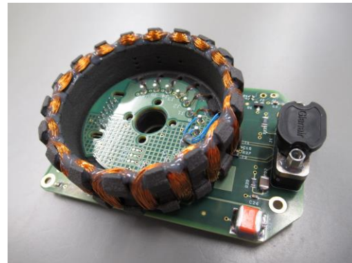
Figure 3: Reaction wheel electronics assembly
