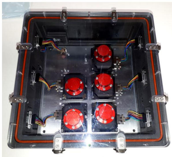
Figure 1: Ground Test Pod populated with five star trackers
