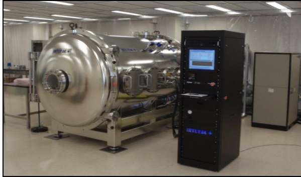
Figure 24: Intlvac Thermal Vacuum Chamber. Dimensions 1.6 m I.D. x 2.25 m long, Vacuum spec: 10-8 Torr.
