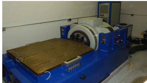
Figure 23: Vibration and Shock Table. Tests objects 1.2m x 1.2m. 5-2200 Hz to 7000 kgf; 14000 kgf shock
