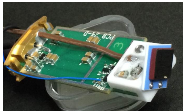
Fig. 1 - CdZnTe detector (CZT) - right hand insert - and its prototype electronic board of acquisition; final electronics developed in house at INPE
