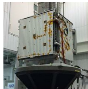
(c) Structural Vibration Test
