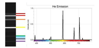
Figure 5: Left, spectral alignment testing using a Helium source. Right, reference image from Vernier.
