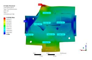
Figure 4: Modeled deformation due to thermal strain from -10 to 30 C temperature change
