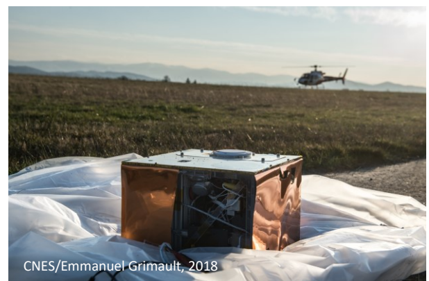
Figure 7: MASCOT spare model and monitoring system during helicopter tests
