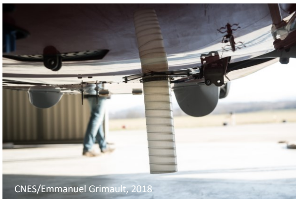
Figure 6: OME-A antenna mounted at the bottom of helicopter cabin
