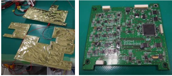
Figure 5: Flight model of CLOTH (left: Smart MLI, right: Circuit board)
