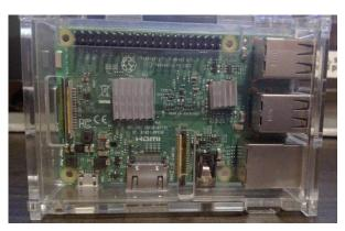
Figura 2.4: Raspberry Pi 3 Model B
