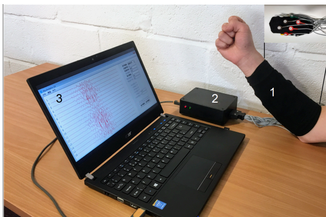
Figure 1. The experimental setup for sEMG data collection.
