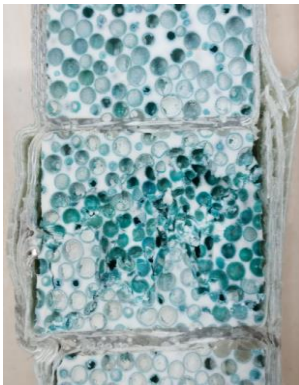
Fig.7 Edgewise compressive failure modes of damaged specimens
