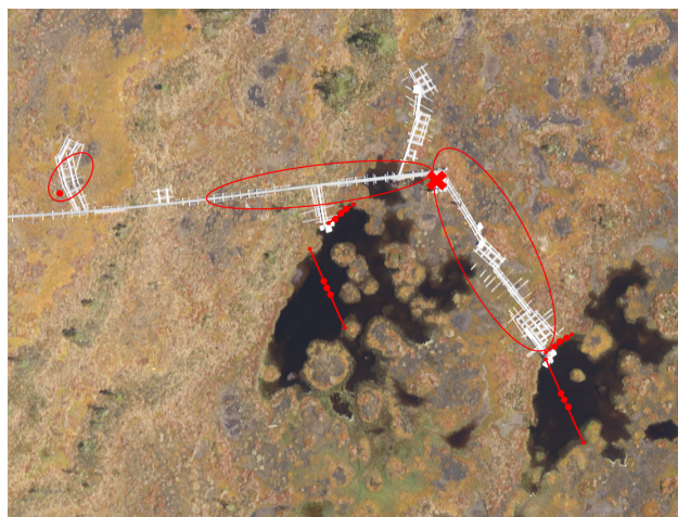
Figure 2. Aerial photo of the study site in Siikaneva bog. Red lines with dots mark the floating gas traps in open water (OW) and at the water's edge (EW). Red circles mark the area where the gas traps were placed on bare peat surfaces (BP), which are seen as brownish-grey in the photo. The eddy covariance (EC) raft is marked with the red \times .
