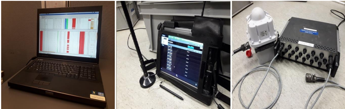
Figure 2. Server laptop, data harvester and battery charger.
