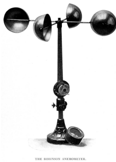
Figure 1: On the left: Hooke's anemometer from 1667 (source: Laughton, 1882) and on the right: Robinson's cup anemometer (source: wikipedia, https://en.wikipedia.org/wiki/Anemometer , accessed: 28.2.2019).
