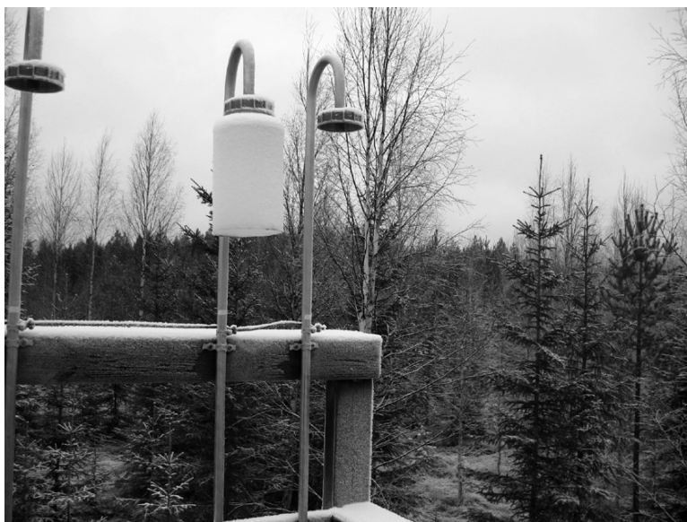
Figure 26: Air sampler for measuring atmospheric gaseous concentration [26].
