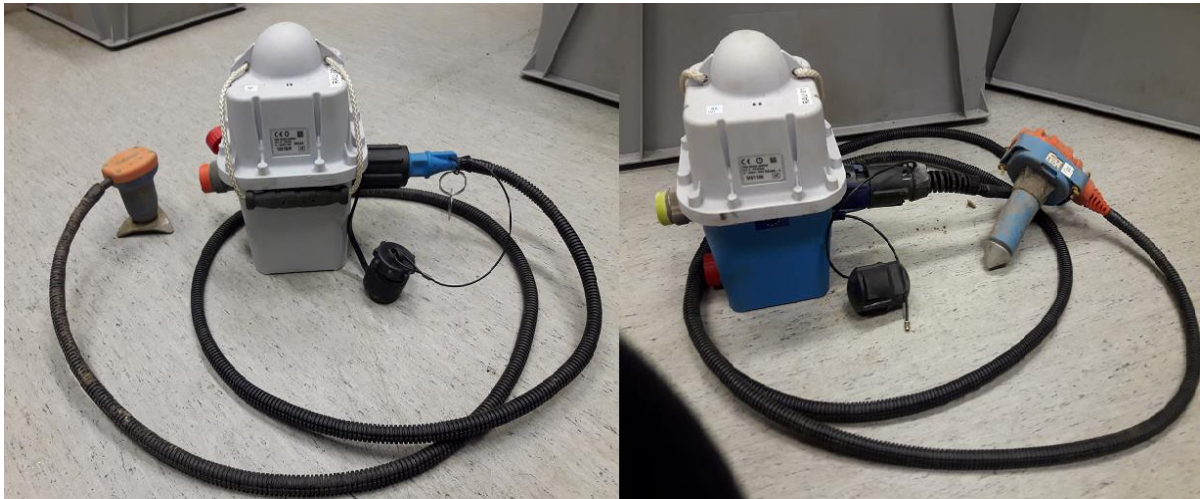
Figure 1. 1C geophone with RAU eX data logger (left) and 3C accelerometer with RAU-D data logger (right).
