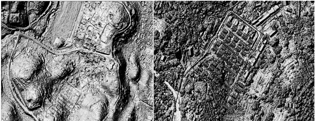
Figure 20. On the left is a DEM, and on the right is a DSM over Wundanyi town, Taita Hills.
