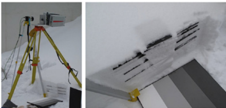
Fig. 3. Left: The snow surface was scanned from above. Right: Metal plates were placed in the snow pack and a Spectralon reflectance panel was placed in the area of the scan.
