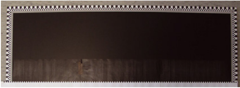
Fig. 1. The plate used as background and scale for the snow surface roughness measurements, here shown in calibration measurements using a print of scaled tooth pattern.
