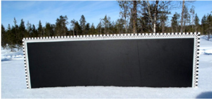
Fig. 4. Validation snow profiles were measured with plate photography by inserting a 1 m wide black plate in the snow. The profiles were automatically extracted from the photographs for deriving snow roughness.
