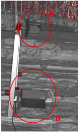
Fig. 2. Intensity image showing the snow sample directly (B) and indirectly through the mirror (A).
