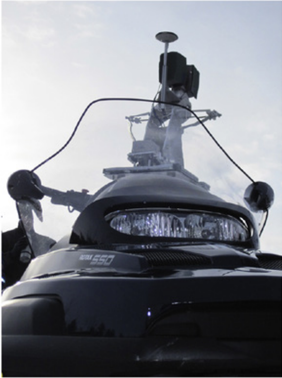
Fig. 2. The ROAMER MLS system and the snowmobile employed for the data acquisition. The GPS antenna and IMU boxes are seen in front of the platform, the laser scanner unit is topped with green insulation.
