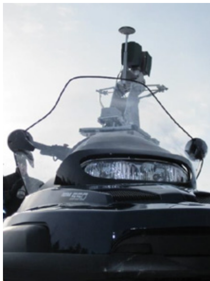
Figure 11 The FGI ROAMER mounted on a sleigh, moved by snowmobile.
