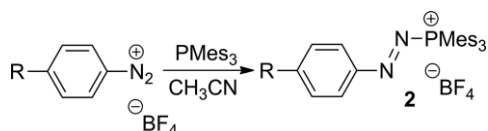
Scheme 2. Synthesis of arylazophosphonium tetrafluoroborates 2 , R = NO 2 ( a ), Br ( d ), H ( f ), MeO ( m ), Me 2 N ( p ).
