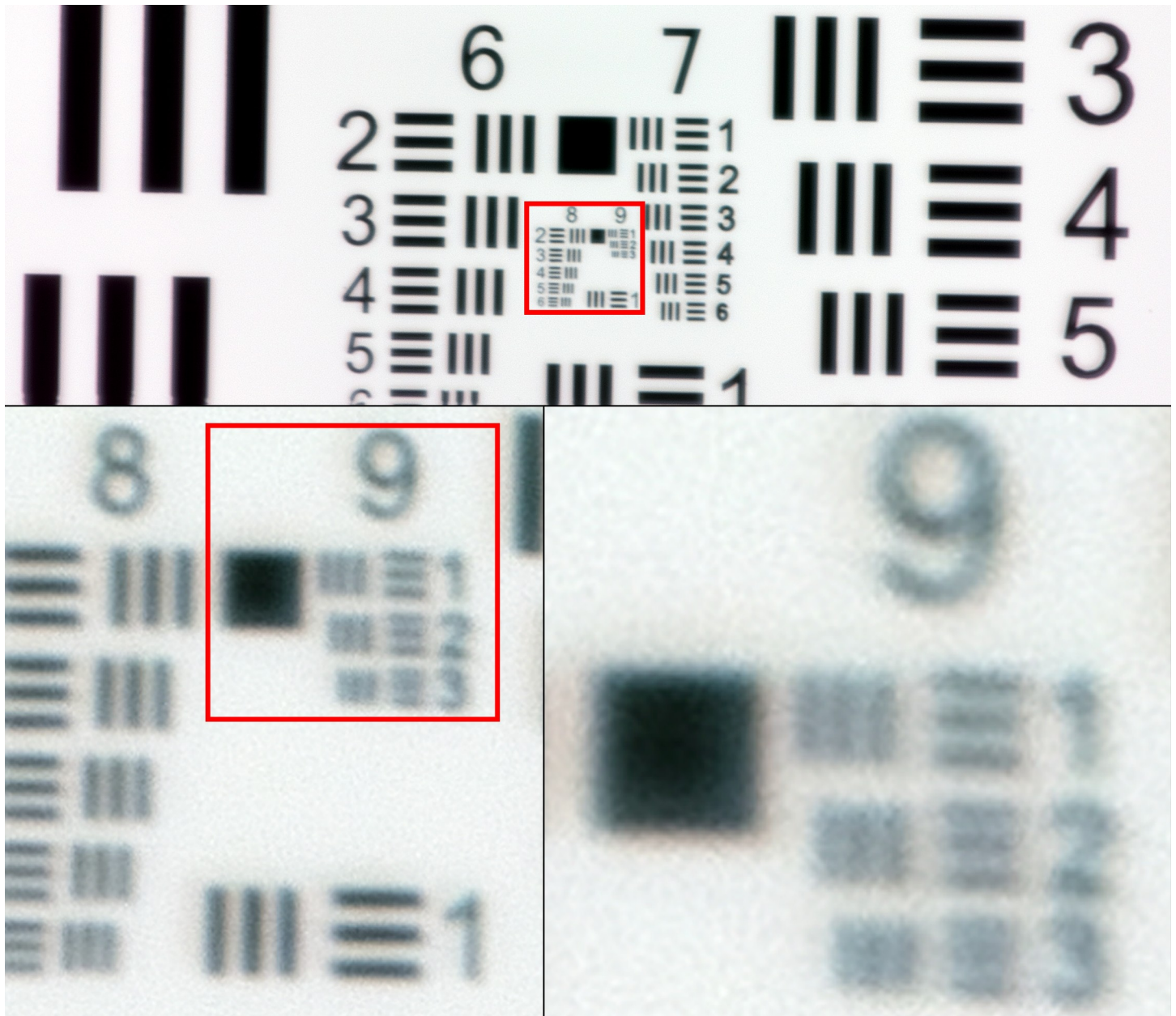
Fig 2. US Air Force 1951 three-bar resolution test chart. Images captured with miniature microscope scanner. Enlarged images showing smallest resolvable bars (group 9, element 2–3), corresponding to a spatial resolution of approximately 0.9 \mu\text{m} .
