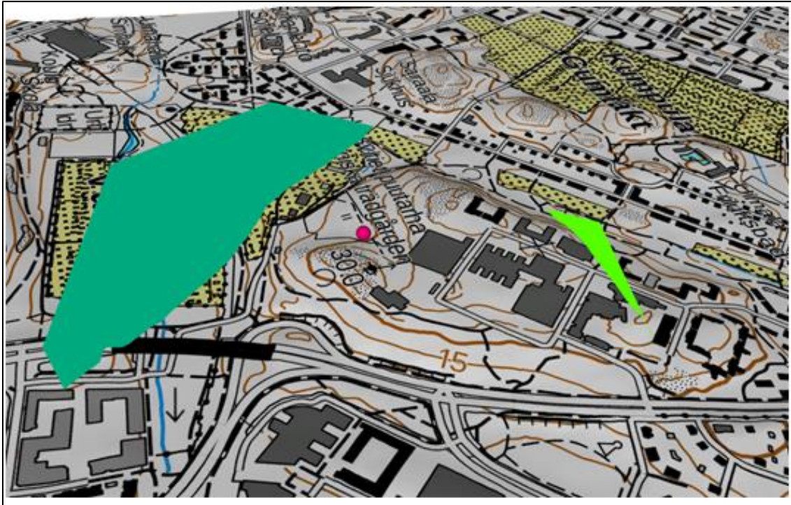
Figure 18. The Kumpula hill from east side. On the left is marked the crushed zone from the depth of 109.0 and on the right is crushed zone from the depth of 296.0. Both are extended from original observation point (from the drill hole) 450 meters in every direction so that they cut with the surface of the ground. The pink point is the place of the drill hole.
