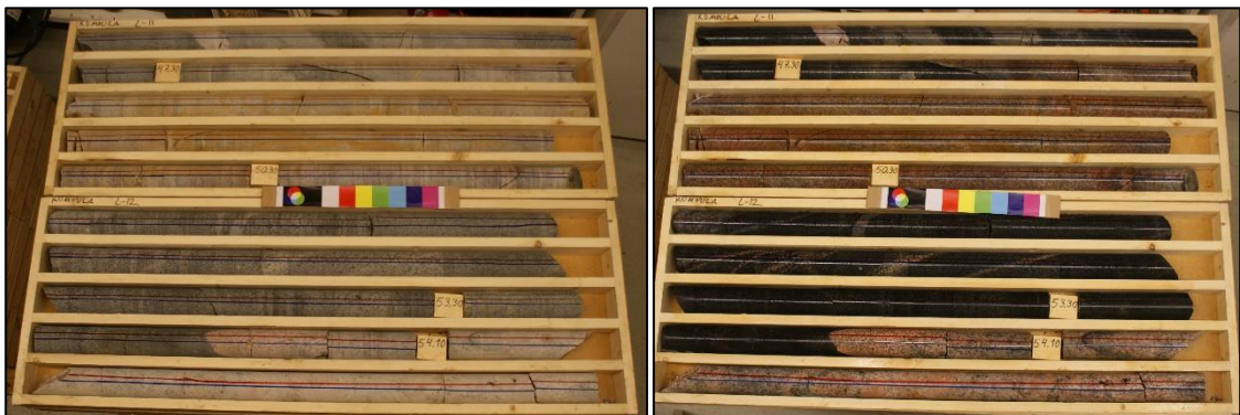
Figure 6. Drill core box number 11 and 12 after drawing accessory lines and before logging, on the left dry core and on the right wet core.
