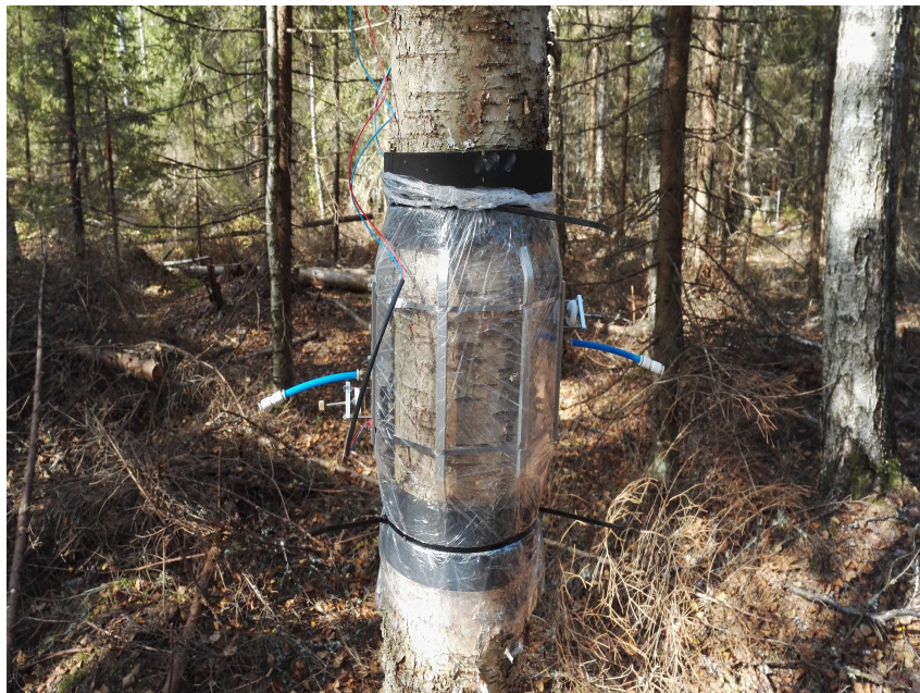
Figure 5: Newer type cylindrical chamber (height: 30 cm, width 2.3 cm)
