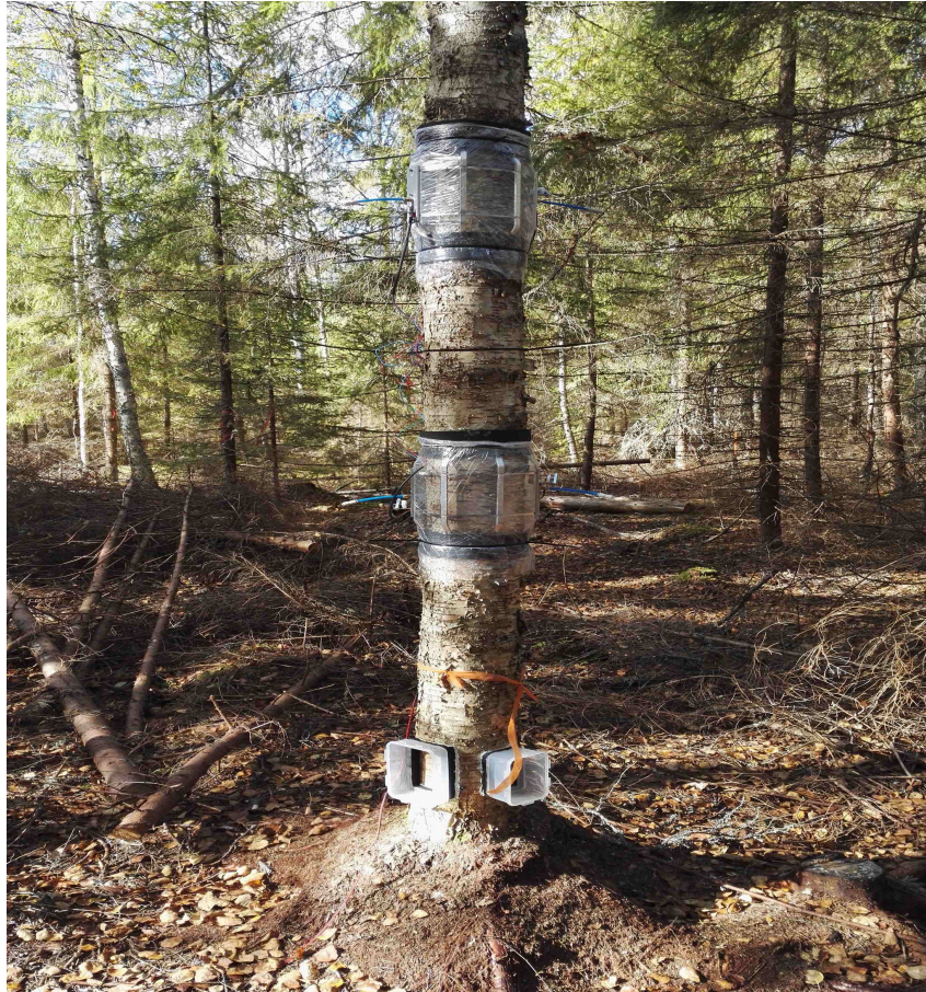
Figure 3: box-shaped static plastic chamber (width: 8.6 cm, height: 13 cm, depth: 6 cm) (lowest in the figure). Also illustrates the profile measurement setup.
