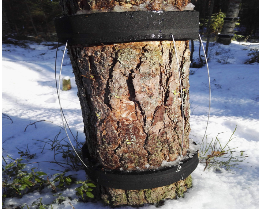
Figure 4: Older type cylindrical chamber without plastic wrap and plate (height: 40 cm, width 4-6 cm).
