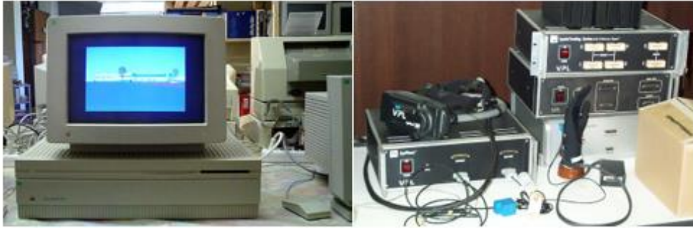
Figure 5. Apple Macintosh II/FX on the left and VPL EyePhone™ and DataGlove™ on the right.
