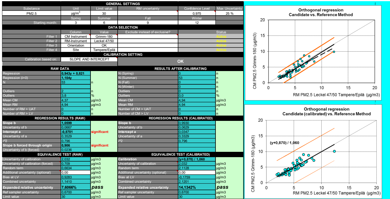
Figure A8a. Verification results in Tampere/Epilä for Grimm-180 (Tampere) in PM 2.5 measurements. Data has not been corrected according to DoE from Kuopio.
