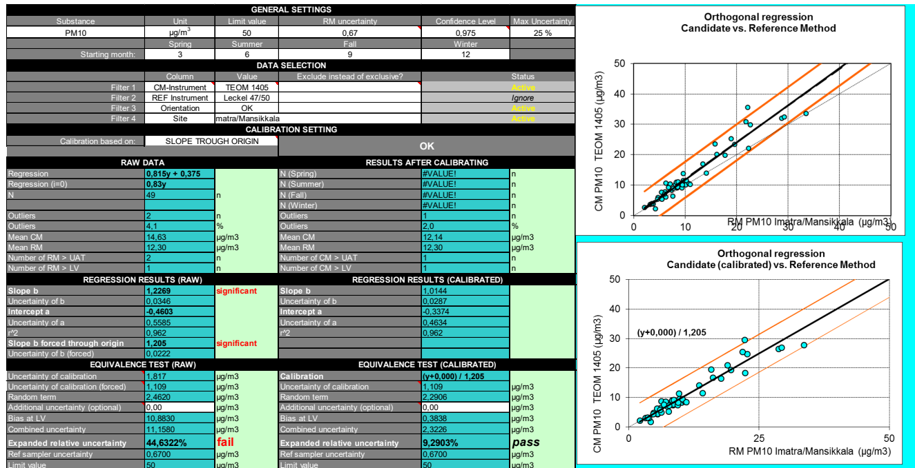
Figure A1. Verification results in Etelä-Karjala/Mansikkala for TEOM 1405 PM 10 measurements. Data has not been corrected according to DoE from Kuopio.
