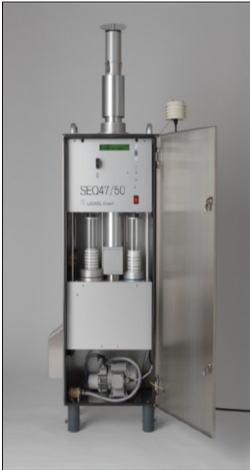
Figure 2.2: The layout of the reference samplers Leckel SEQ 47/50 (left), and Derenda PNS (right) used for the PM_{10} and the PM_{2.5} verification tests.
