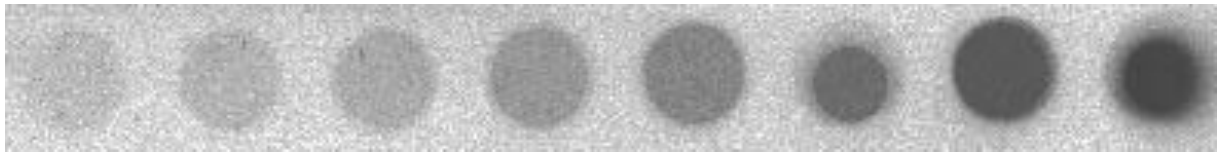
Figure 8. A calibration standard series with known activities (lower activities on the left, higher activities on the right)
