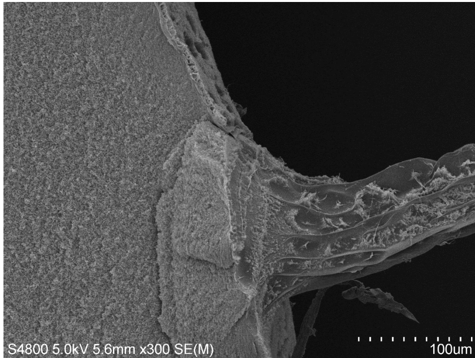
Figure 59. SEM image of a FCB bead. The base of the tail is shown in cross-section while the tail itself is left whole.
