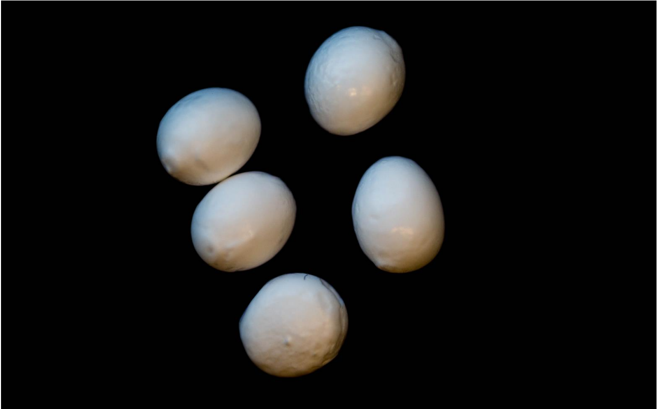
Figure 46. These Freeze-dried Cellulose Beads (FDCB) have an oval shape to them and the surface of the beads is also somewhat uneven. The diameter of the beads is ca. 2 mm.
