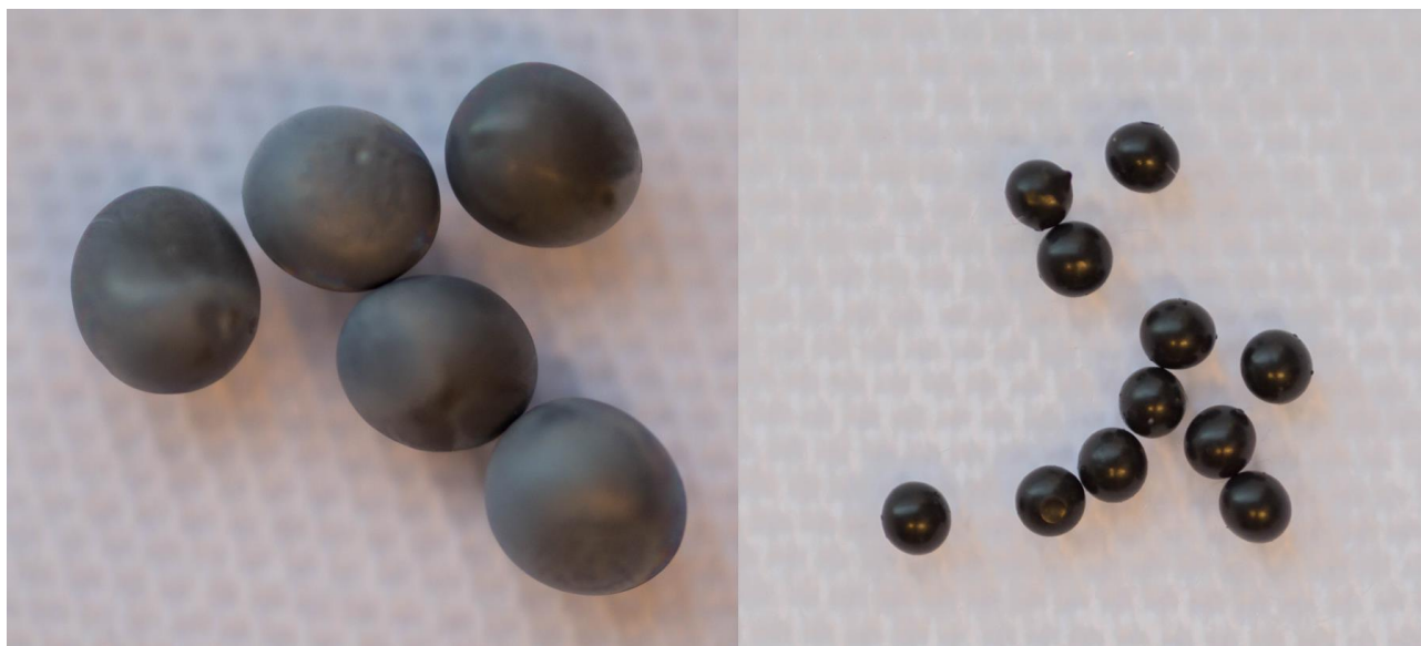
Figure 50. Freeze-dried and air-dried cellulose beads containing 20 wt-% iron powder.
