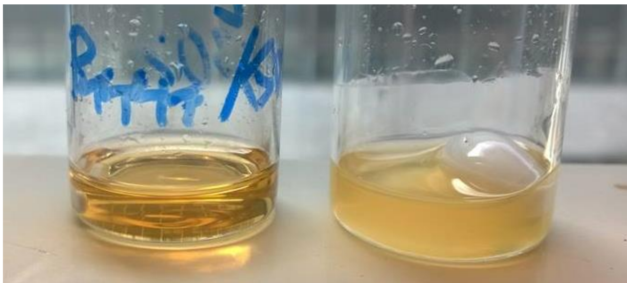
Figure 62. Comparison of the 1 wt-% (left) and 4 wt-% (right) UCST dopes after 24 h storage in the refrigerator. The presence of at least partially precipitated cellulose is indicated by the opaqueness of the 4 wt-% solution.
