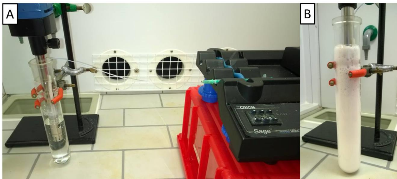
Figure 40. A: The setup used to test nanoprecipitation while mixing with Ultra-Turrax mechanical mixer. The syringe is connected by a flexible tube to a needle taped to the shaft of the Ultra-Turrax mix head. B: Excessive foaming resulting from the presence of 1 wt-% of Aerosol OT surfactant along with cellulose in the [DBNH][OAc]/DMSO-dope. The intensity of mixing had to be reduced to avoid further foaming.
