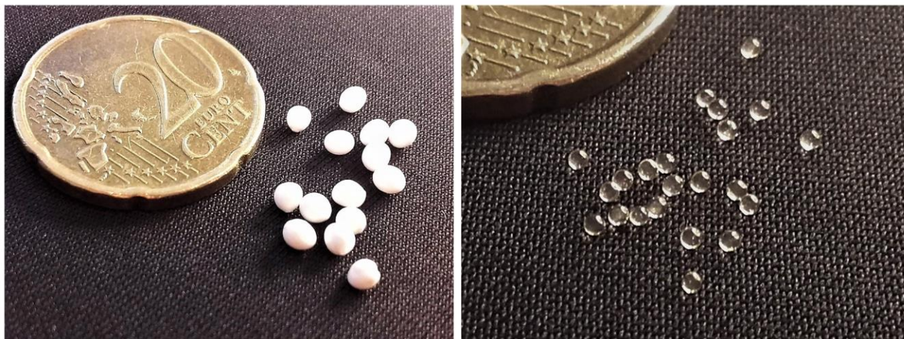
Figure 43. The freeze-dried Cellulose Beads are large (diameter ca. 2 mm), porous and opaque, while the air-dried Cellulose Beads are small (diameter <1 mm), dense and transparent.
