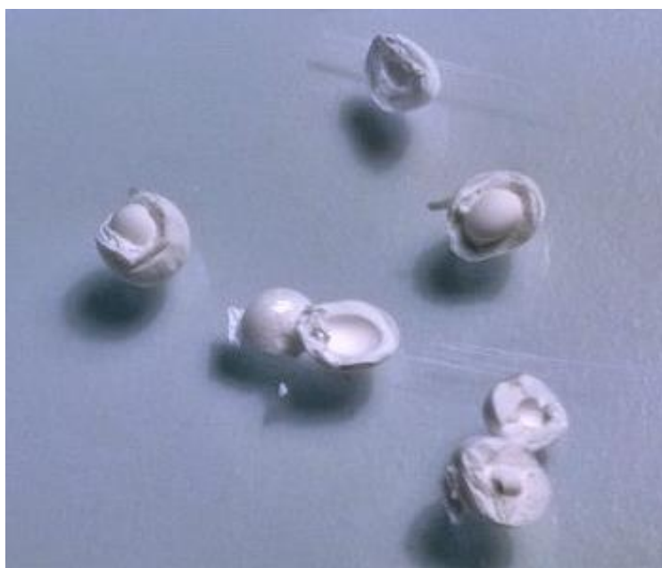
Figure 53. Split FDCB beads displaying the variation in the core-crust ratio.
