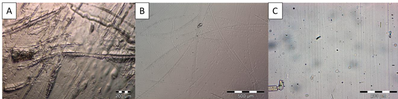
Figure 36. Optical microscope images of the cellulosic dialysis bag used in the dissolution and dialysis tests. A: 10 mg piece of dialysis bag immersed in [P_{4441}][OAc]/DMSO for 24 h, B: 10 mg piece of dialysis bag immersed in [P_{4441}][OAc]/GVL for 24 h, C: piece of the dialysis bag used in a dialysis test using [P_{4441}][OAc]/GVL as the sample to be dialysed.
