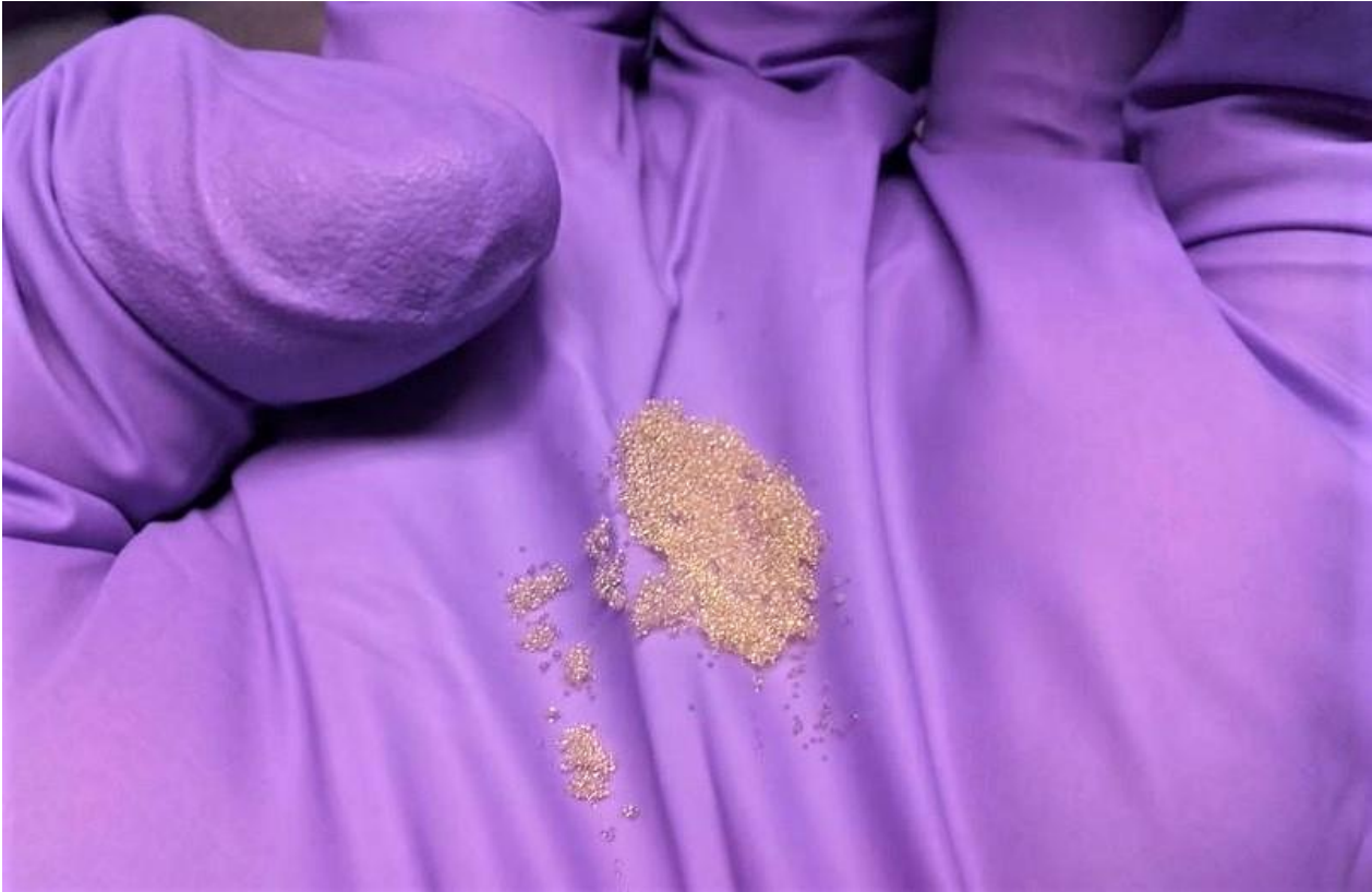
Figure 19. Plastic microbeads between 300 and 600 \mu\text{m} in diameter, consisting of styrene-divinylbenzene copolymer.
