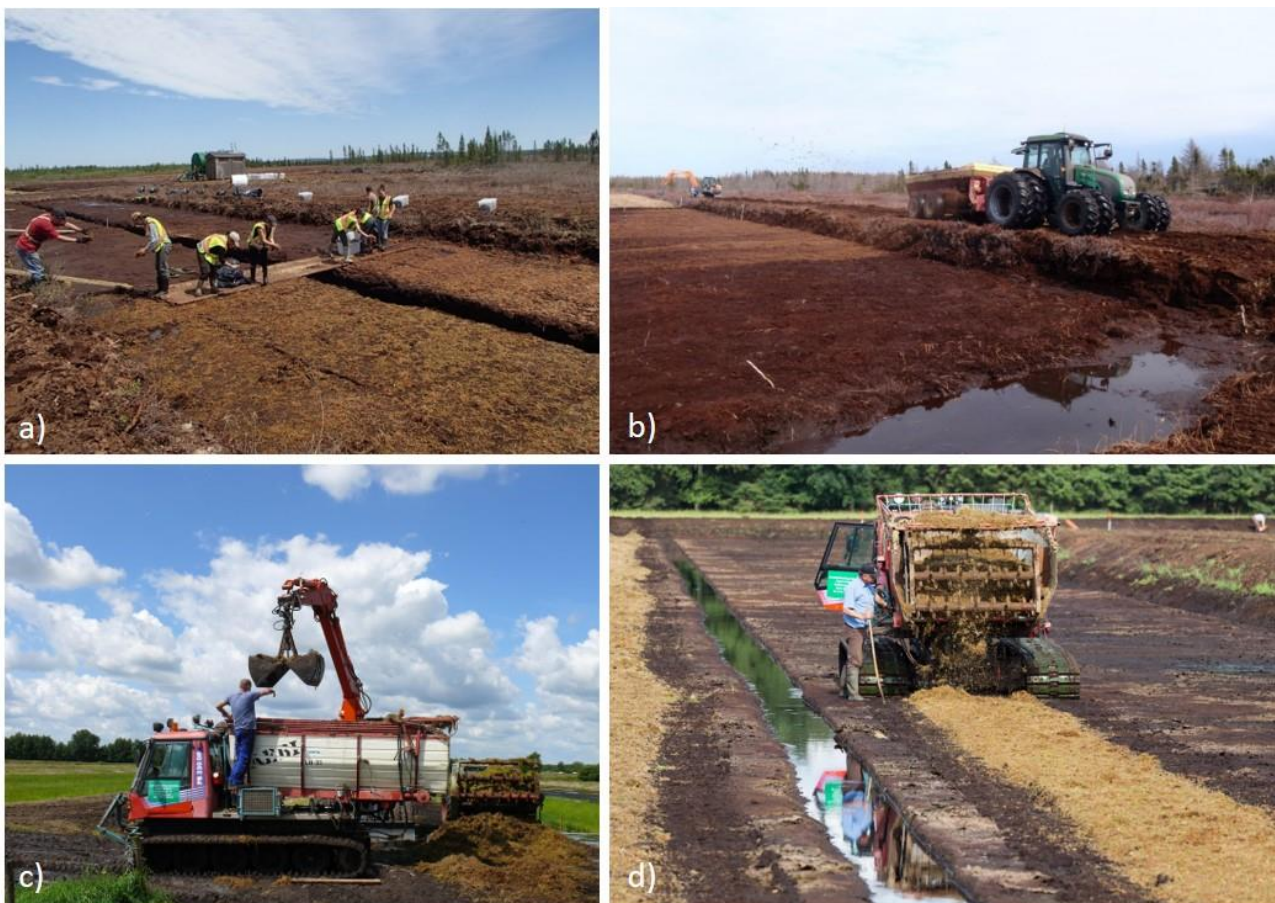
Figure 5. Spreading of Sphagnum and straw mulch: a) manually; b) mechanically by a tractor driving along the edge of the field pulling a manure spreader or a machine that blows the straw onto the site; or by c) loading founder material onto a manure spreader mounted on a tracked vehicle which then d) drives directly on the field. Photos: a) and b) Peatland Ecology Research Group, c) Sabine Wichmann and d) lensescape.org.
