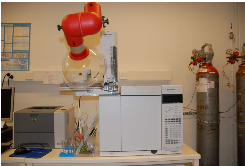
Kuva 5 Gas chromatography (GC) was performed using an Agilent 7890A instrument equipped with a flame ionization detector (FID) and Agilent 7683B autosampler.
