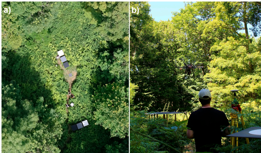
Figure 5. (a) An aerial image of the take-off and landing site. The reference panels BC, GC and GP in direct sunlight and in shadow are visible in image. (b) An image of the UAV landing site. The proximity of trees to the reference panels is evident in this image.
