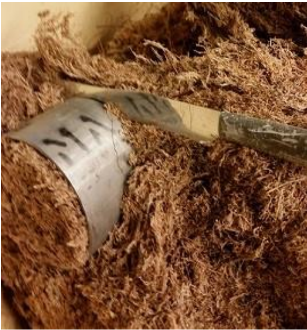
Figure 2. Cutting of the attaching fibres after driving a soil sample cylinder into a Sphagnum bale.
