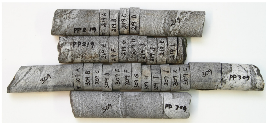
Fig. 1. The sawed rock samples of drill cores PP219 and PP309. The samples 219A, 219D, 219H, 219L, 309A, 309D, 309H and 309L were used in the electromigration sorption experiments of cesium. The electromigration of strontium was studied with the samples 219B and 219E. The rock slices 219F, 219J, 219K, 309F, 309J and 309K were used in the determination of minerals by the thin section method. The rest was crushed and sieved for the batch sorption experiments and specific surface area measurements (Lehto et al., 2018).
