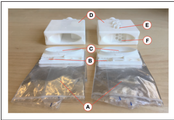
Figure 2. Photo of the active device (left) and the sham device (right), showing (a) the folded rebreathing reservoirs; (b) bypass valves; (c) reservoir connectors, shown dismounted from mouthpiece boxes (d); (e) sham device airflow redirection holes, with protruding structure for preventing accidental blocking by fingers, (f) sham device one-way check valve.
