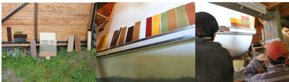
Figure 11. Paint selection process. Left: matching colour plates in daylight. Center and right: matching colour plates on the side of the ship.
