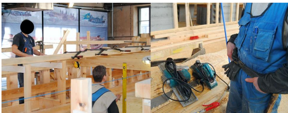
Figure 7. Working on the gunboat. Left: division of labour between the shipwright and an apprentice: the shipwright is conducting the measurements, while the apprentice is fixing/placing the clamps in place. Right: the shipwright is showing his instruments to the apprentices.
