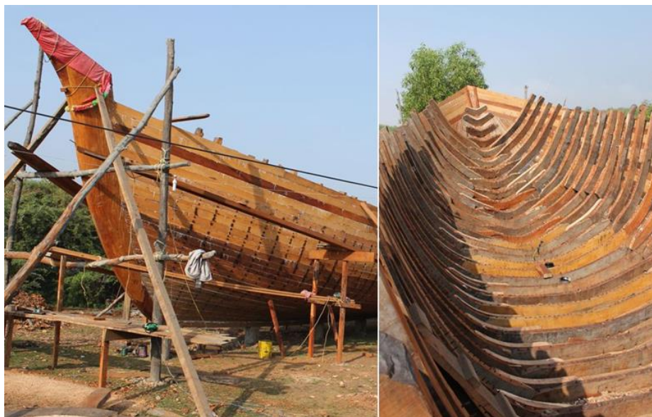
Figure 22. Shape of the hull and the construction process when using the skeleton-based technique: Indian site.
