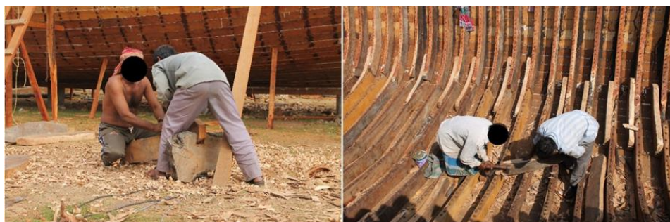
Figure 14. Working on the ribs. Left: cutting ribs outside of the hull. Right: installing the ribs.
