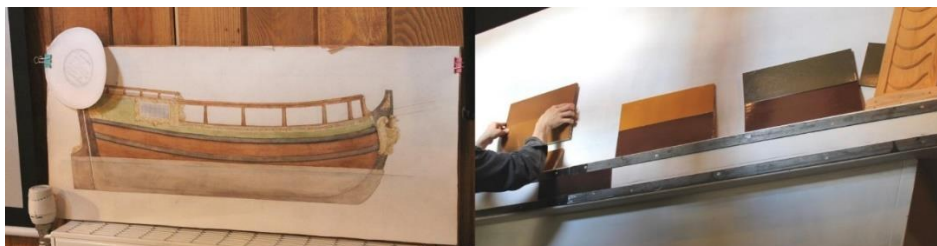
Figure 32. Colour choice at the Russian shipyard. Left: colour sketch of the ship. Right: choosing colour combinations with the help of painted wooden plates.
