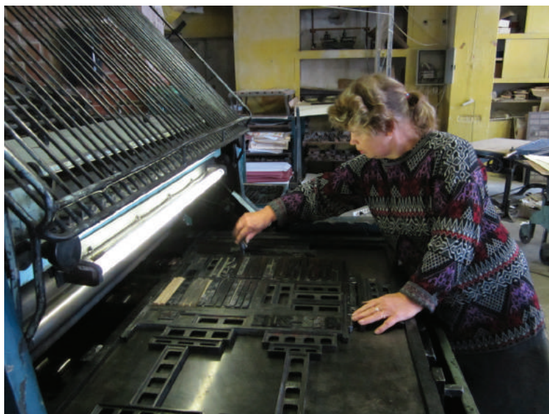
Fig. 2.8 Ljuda using the Victoria 1040–2 typesetting machine. Source: Author, 2013.
