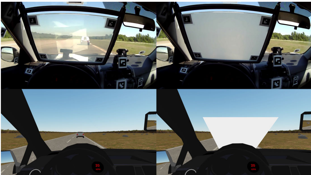
Figure 5. Participant view in the real car (top) and VR simulator (bottom) CF experiments with the occluder off (left) and on (right).
