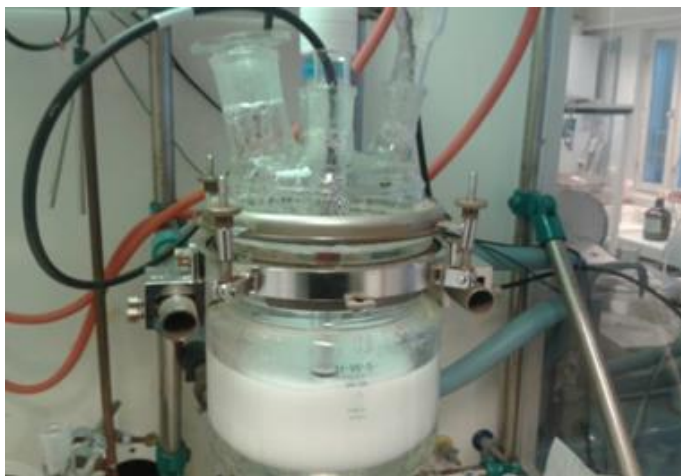
Figure 4. Huber reactor (3 L) equipped with water bath used for preparation of \alpha -ZrP
