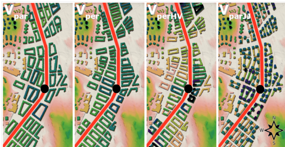
Figure 1. The city-block-design alternatives. From left to right: V_{\text{par}} (the longer sides of buildings parallel to the boulevard), V_{\text{per}} (the longer sides perpendicular to the boulevard), V_{\text{perHV}} (similar to V_{\text{per}} but the building height varies) and V_{\text{parJJ}} (similar to V_{\text{par}} but with Jing-Jang building structure variation). The boulevard is marked in red and the major junction with a black dot.
