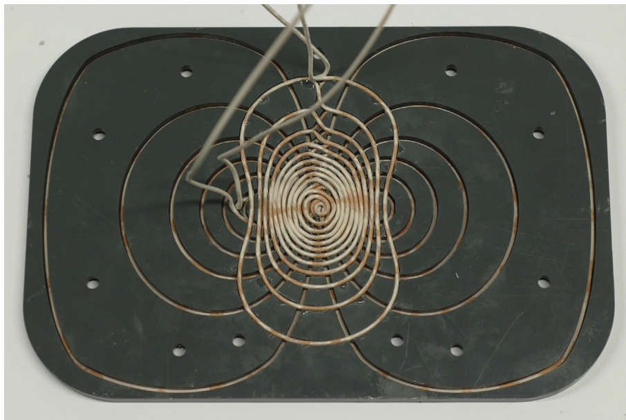
Fig. 2. Two-coil mTMS transducer. Our transducer consists of a minimum-energy figure-of-eight coil and an overlapping oval coil. The figure-of-eight coil alone produces a focal stimulus underneath the centre of the transducer. The oval coil alone produces a relatively broad stimulus on both sides of that location, with the E-field reversing its direction underneath the centre of the transducer. As a superposition of the fields of the two coils, we obtain a focal stimulus to the desired target near the centre. After the photograph was taken, the wires were glued in place with epoxy.
