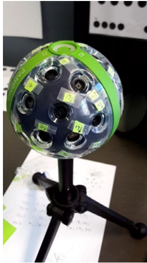
FIG. 3. The Panono camera; all 36 projective cameras are individually labelled.
