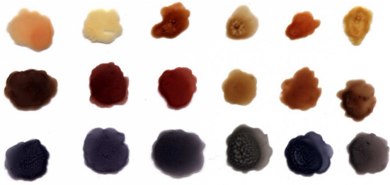
Figure 4: Paint mixtures that are usually pairwise mixed to form the color for each layer.
