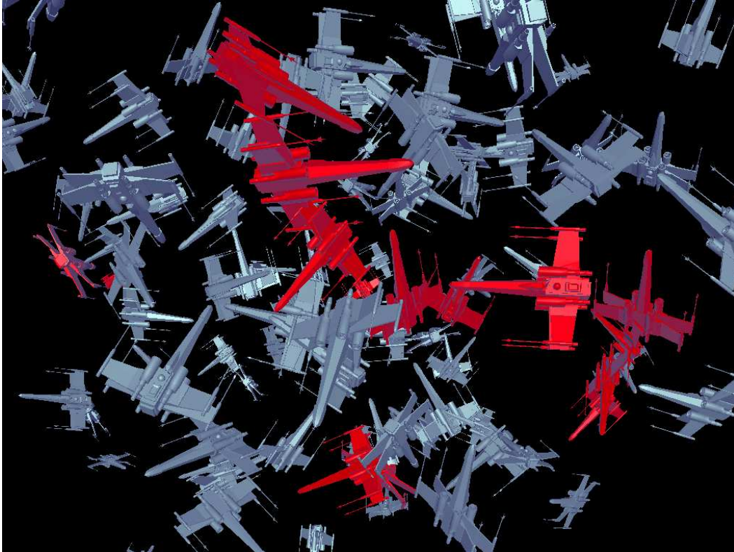
Fig. 6. Example of a complex model scenario requiring kinetic sweep and prune, along with OBB-trees for efficiency. Each of the 100 models is composed of over 6000 triangles, for a total of over 600,000 triangles; our collision detection engine sustains over 15 frames per second, including dynamic intersection tests. Red models are colliding.
