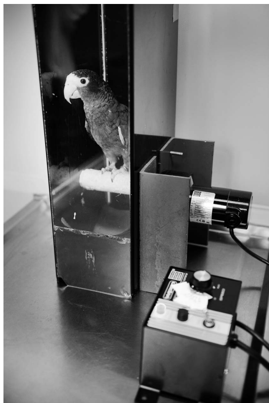
Figure 1. A rotating perch was used to provide walking exercise for Hispaniolan Amazon parrots. The apparatus consists of an opaque acrylic box with a clear front panel and a nonskid perch connected to a direct current motor, with a variable speed control box. The speed was adjusted to maintain a brisk but sustainable pace for the parrots, which was less than the maximum speed attainable for the apparatus.
