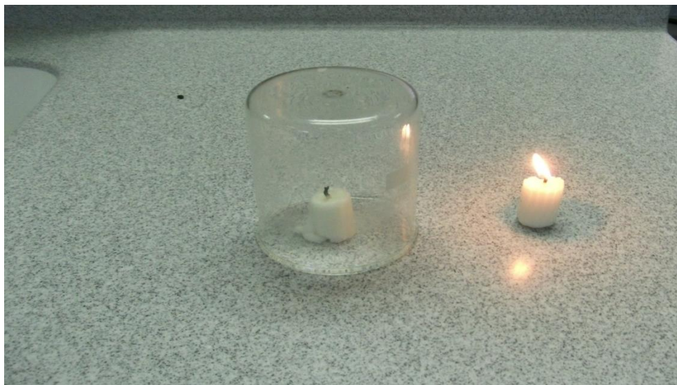
Figure 6.2.1.2: One of the burning candles was covered with a beaker, limiting the access of air to the burning candle
