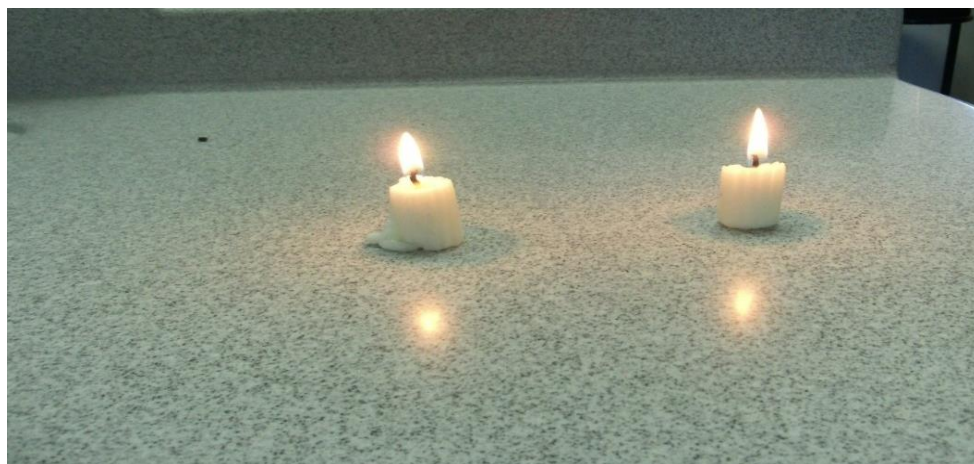
Figure 6.2.1.1: Both candles were burning, having supply of air and fuel (nothing was limiting the combustion)
