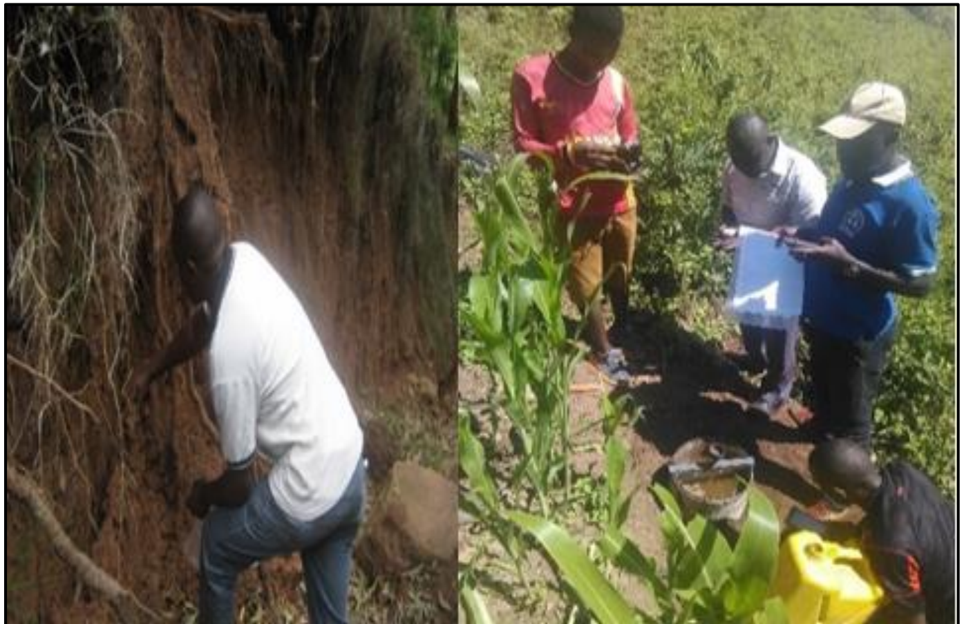
Fig. 4.1: Field analysis of soil properties in the mini-pits, profiles and infiltration tests.
