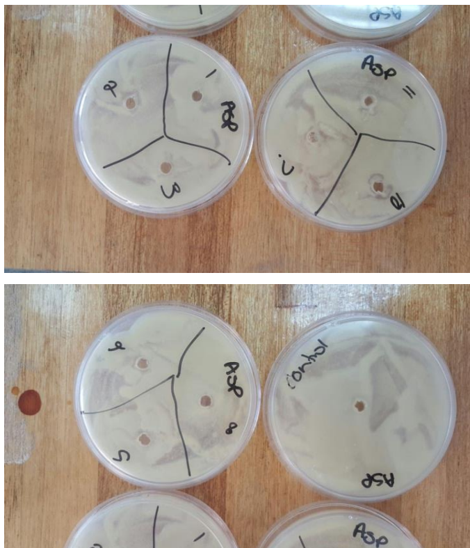
Figure 6.8 Inhibition zones after inoculation with Aspergillus niger : Samples 1, 2, 3, 5, 6, 8 are Coratina extracts; samples 9, 10, 11 are Frantoio extracts
