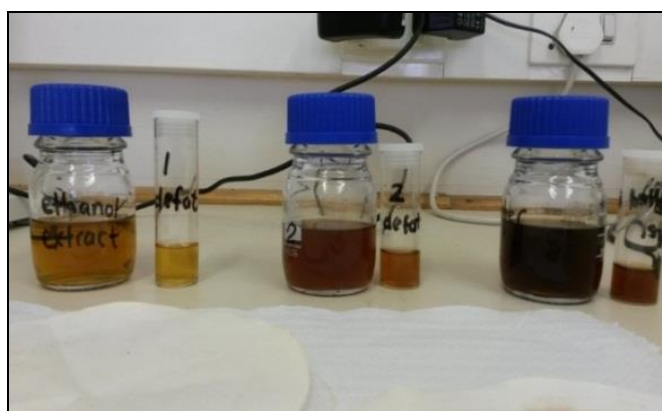
Figure 4.3 Appearance of first three extracts obtained before and after filtering: 1 – ethanol extract; 2 – 50% aqueous ethanol extract; 3 – water extract.
