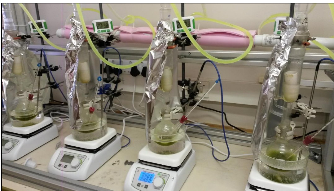
Figure 5.5 Extraction manifold of four Soxhlet units with thermometers inserted into the solvent flasks and probes in the water-bath.
