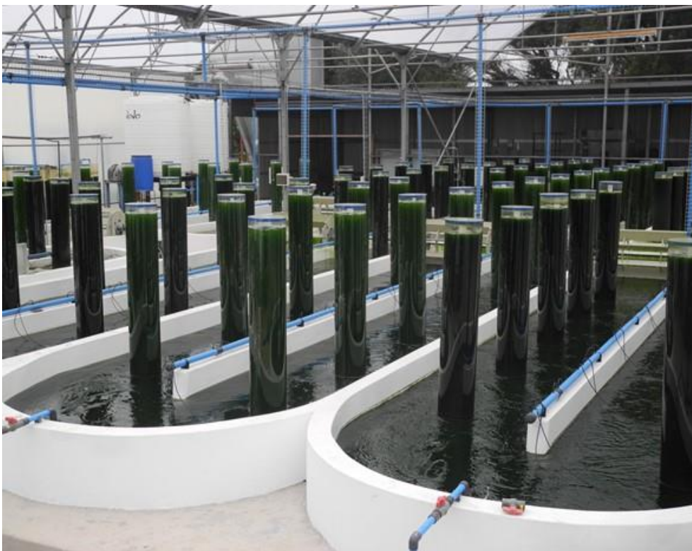
Figure 2.2: Photobioreactor for cultivation of microalgae, InnoVenton
