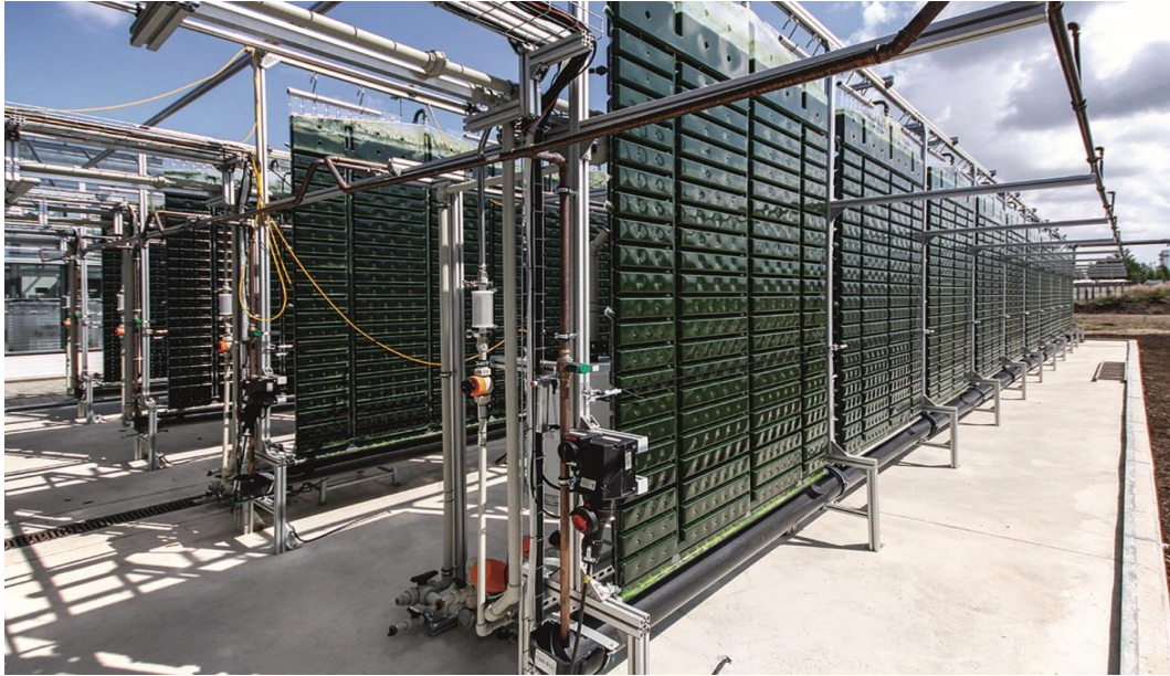
Figure 1.9: Commercial photo-bioreactor for Microalgae cultivation (97)
