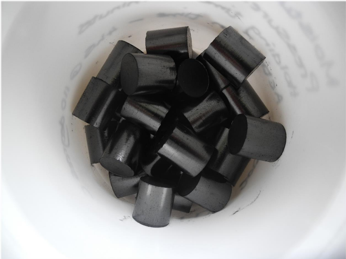
Figure 3.1: Coal-microalgae biomass pellet, “Coalgae®” from blends
