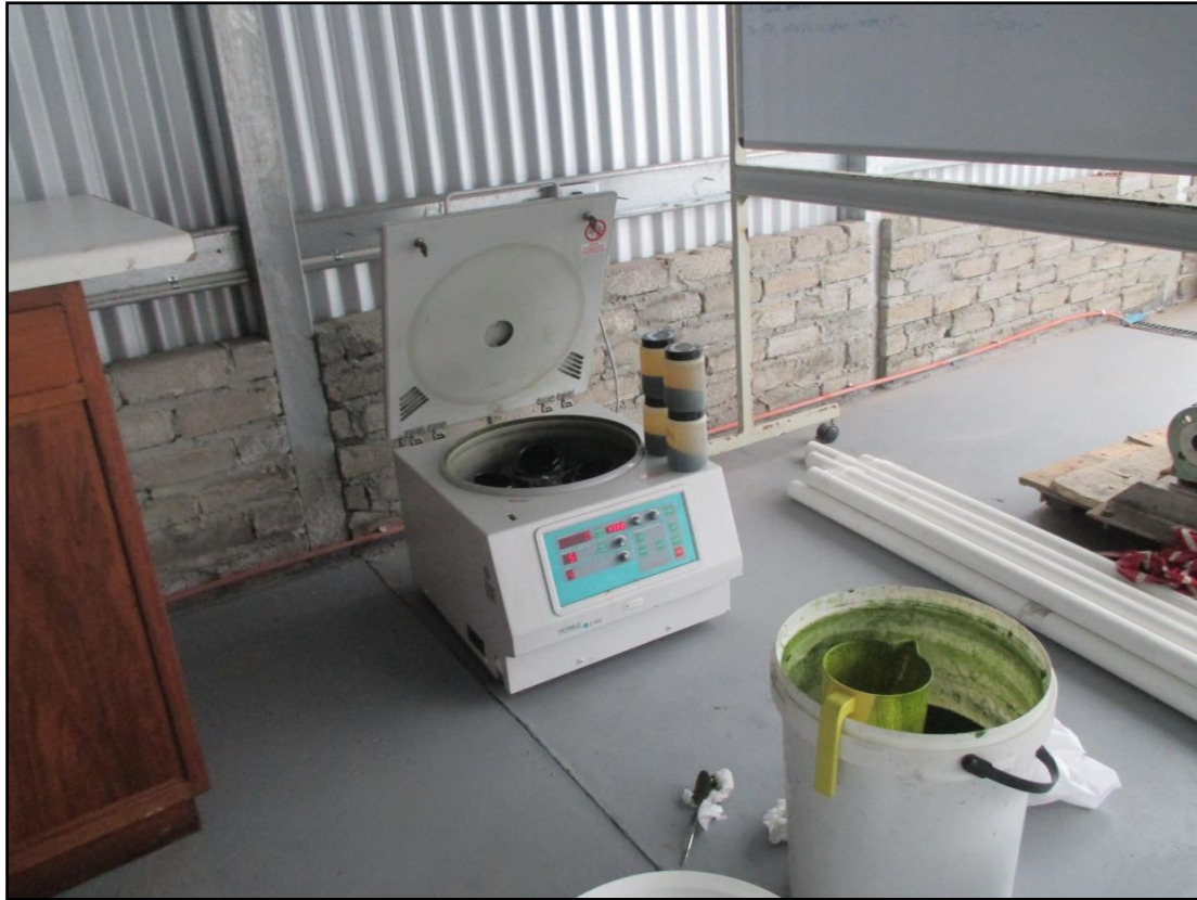
Figure 2.3: Dewatering and cleaning of microalgae biomass with centrifuge
