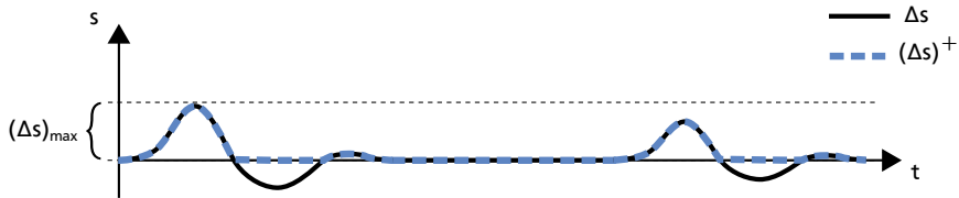
Figure 3.24.: Common exemplary progress of the position error after manual brake input and visualization of investigated variables (\Delta s)^+ and (\Delta s)_{max}
