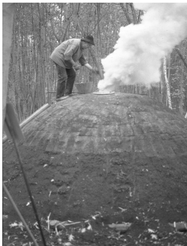
Figure 3: Through the chimney, from the top, wood and/or bad quality charcoal from the previous combustion is regularly added, and fresh pure clay is frequently added to cover the mound.
