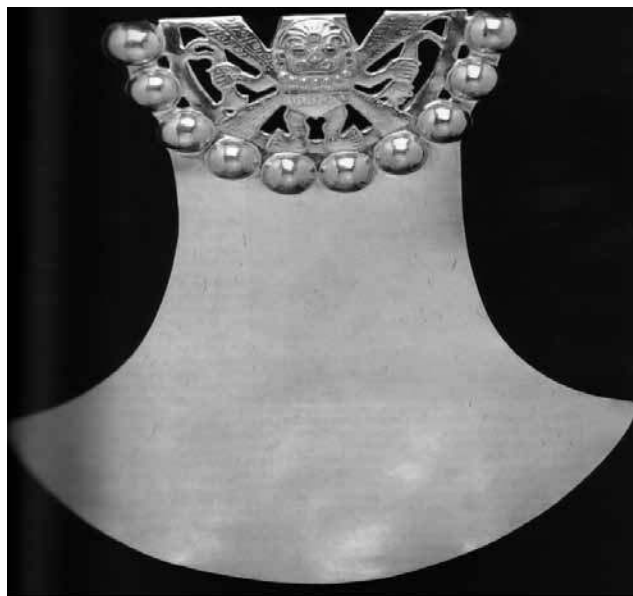
Figure 5: Leg protector made of tumbaga . The ratio Cu(K \alpha /K \beta ) is 4.8, corresponding to an Au thickness of 3.1 \mu\text{m}
