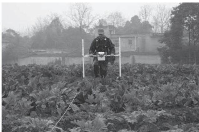
Figure 1: Typical ground conditions for archaeological survey in the Chengdu Plain. The Bartington Grad601-2 dual fluxgate gradiometer is shown here being carried through a field of dense vegetables. The low earthen bank of a paddy wall can be seen running across the foreground.
